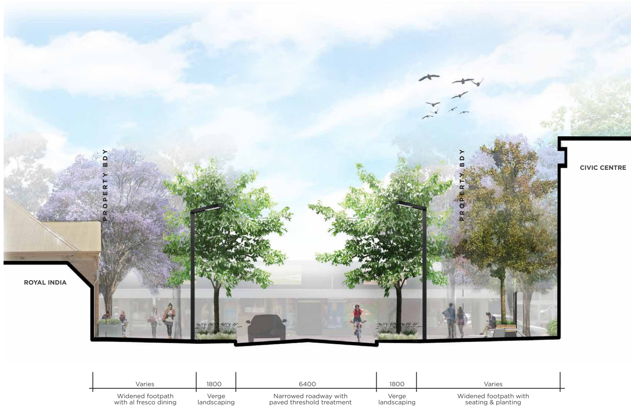
Section C - Norman Street threshold section
